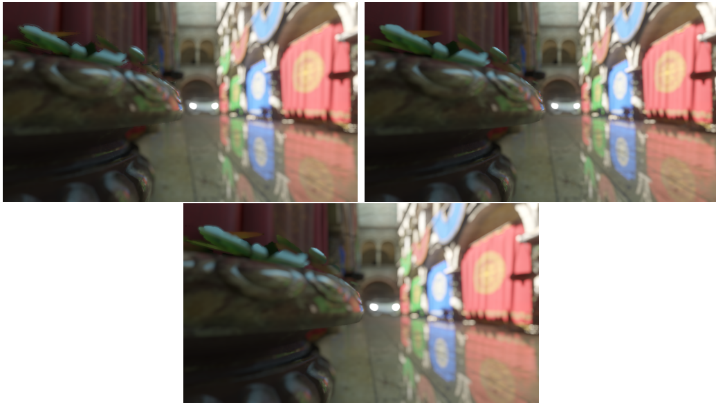
Fig. 4.2. Simple depth of field (top left), sprite based depth of field (top right) and scatter-as-gather depth of field (bottom) applied to the first test scene.
