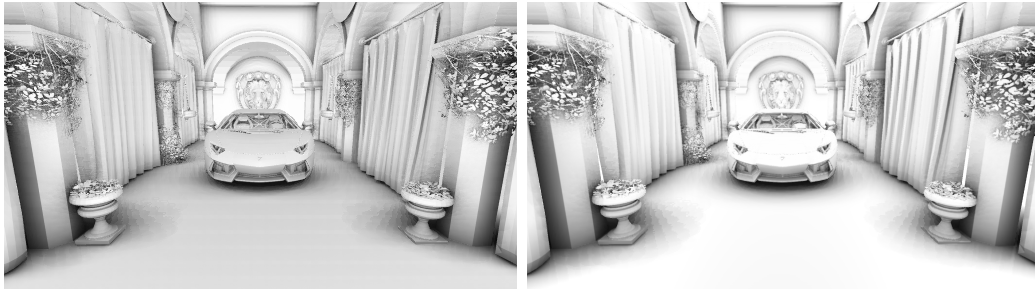
Fig. 3.27. Without the spatial noise reduction, the noise pattern is clearly visible (left). The result of this operation (right) still needs to be filtered temporally.
